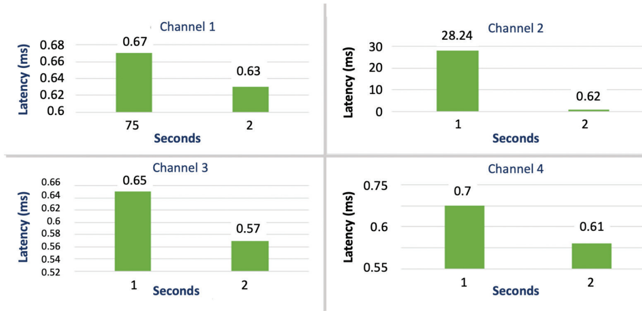
Fig. 12. Evaluation of block interval (1s and 2s) for TPS = 75 (Tables 11 and 15) in Write operation with the number of channels increase from 1 through 4. TPS: transactions per second.
