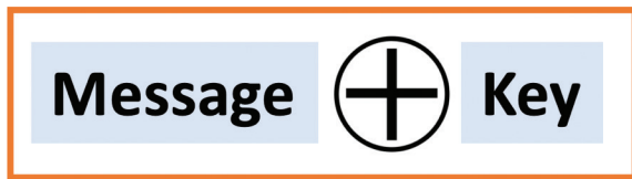
Fig. 4. Encryption procedure by using the first part of the key.
